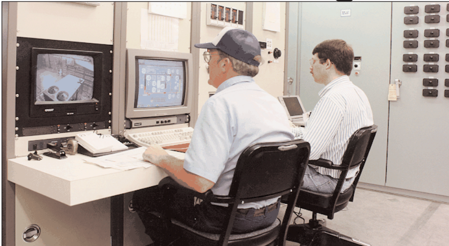
◀ The video screen on the left allows the lab technician a live view of the actual unit while it is being tested.
